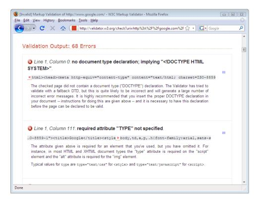
Figure 8.16. Highlighting and explaining validation failures
